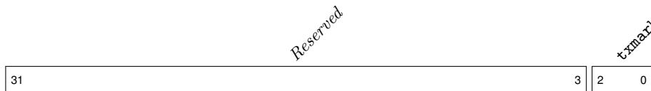
Figure 13.11: Format of txmark register.
