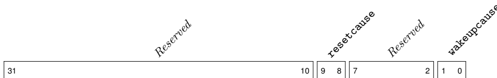
Figure 6.4: Format of pmucause register.
