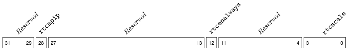
Figure 9.2: RTC counter register pair rtchi/rtclo
