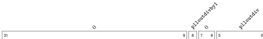
Figure 4.3: PLL Output Divider Register plloutdiv
